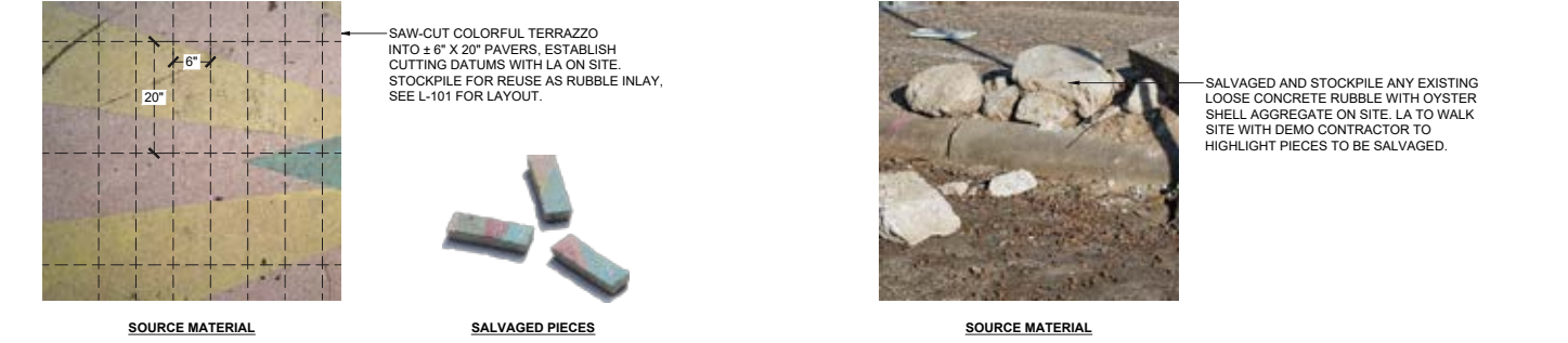
4 COLORFUL TERRAZZO NTS 5 EXISTING CONCRETE RUBBLE, OYSTER SHELL AGGREGATE NTS
